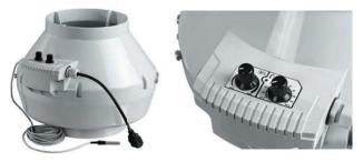
GI – temperature and speed controller with a sensor built into the fan casing. The fan is equipped with a power cord with a socket or plug (GI1). G and GI options are used for automatic speed control depending on indoor temperature. The best ventilation solution for premises requiring permanent temperature control as greenhouses, orangeries, etc.
